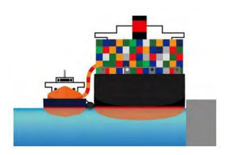
(From left to right : LNG Bunkering vessel, LNG Fueled vessel)
