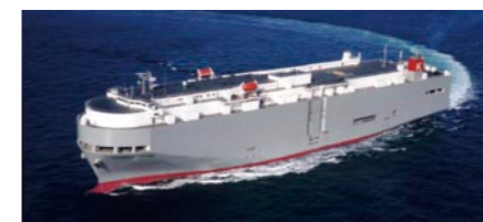
Heat shield paint is highly effective for a car carrier because the accommodations and upper part of the bridge are wide.
